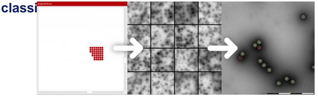
Automation is enabled by using a pre-configured MiniTEM software script, easily designed by dragging and dropping building blocks.
