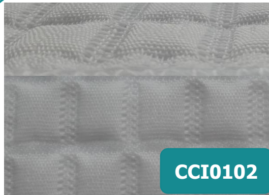
3D woven fabric with insert weft
