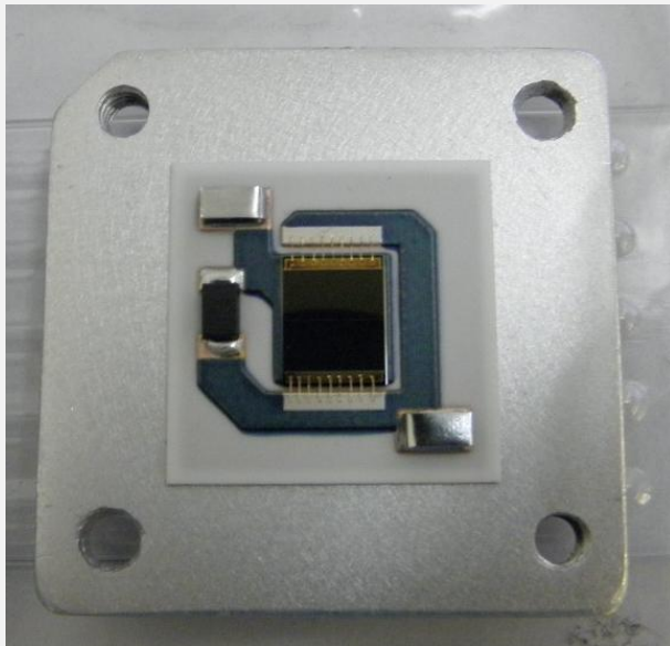
CPV receiver developed and realized by ELCERAM with close collaboration with UWB.
