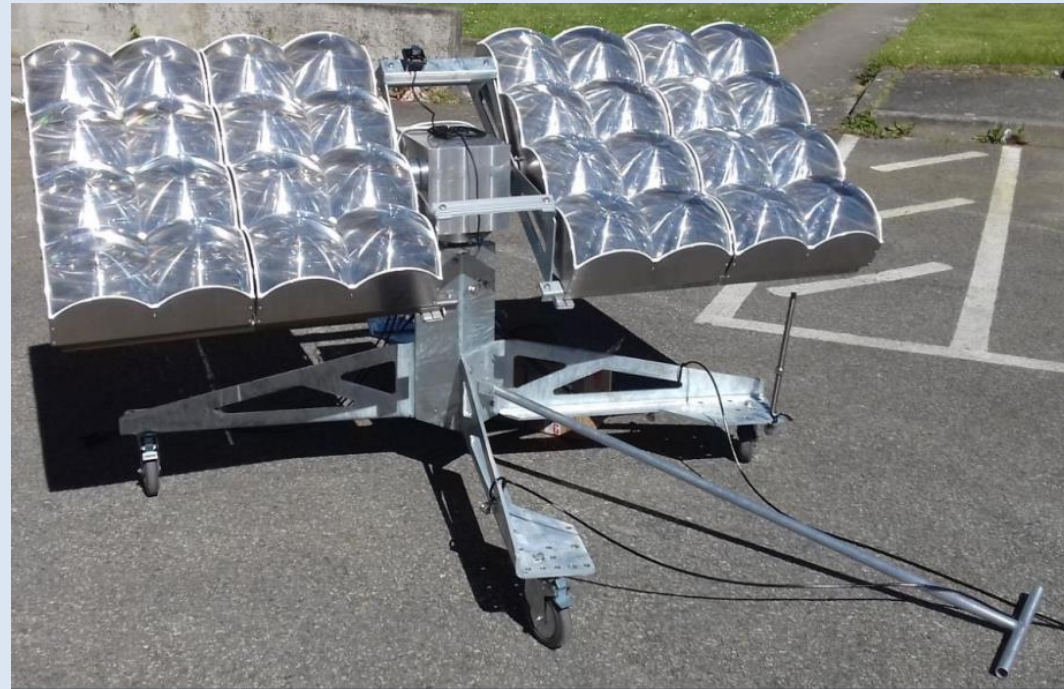
The complete ASES CPV system (25% of efficiency at the CPV outputs).
